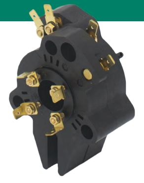
Slip ring collector, consisting of rings coupled with brushes, designed for small jib cranes. Compact sized and equipped with 4 rings.
